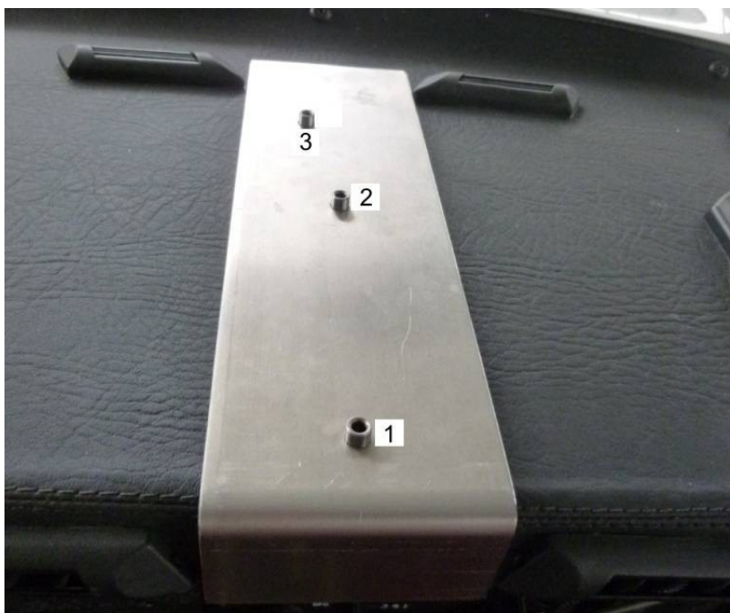
Figure 7 Drilling Template on the glare shield
