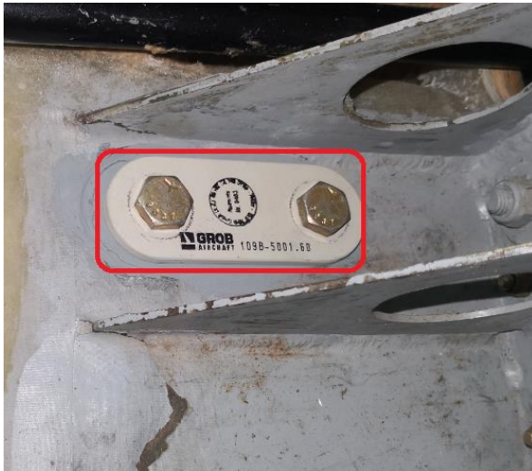
Figure 2 Bracket inside the fuselage
