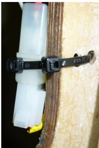
Figure 10 Connectors tied to aircraft frame
